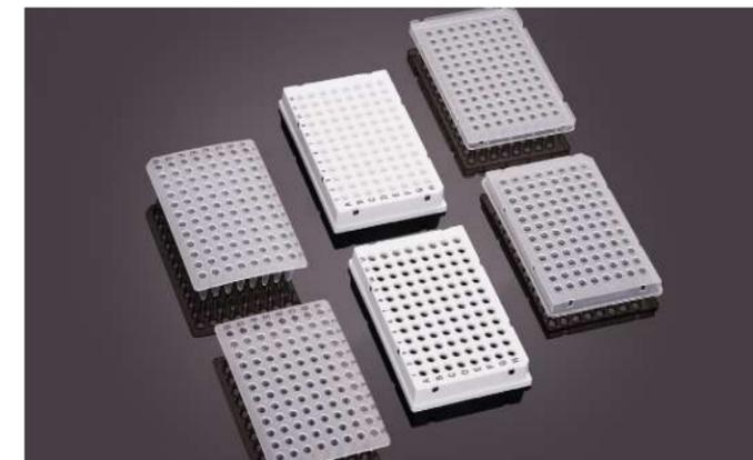
96-Well, flat top PCR microplate is designed to fit standard 96 well blocks. Ultra-thin and consistent wall thickness allows precise thermal transfer for optimum results. Can be sealed with 8/12 strip caps, or sealing film.
