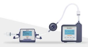
CR-4 with an air sampling pump Accura 2, external filter CR-44 and dumper
