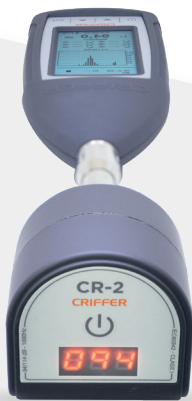
CR-2 calibrating the Sonometer Octava Plus in 94 dB, 1000 Hz
