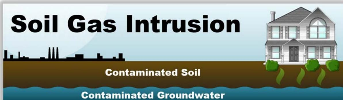
Soil gas/vapor intrusion happens when VOC/SVOC in the air matrix space of soil find their pathway into a buildings, whether residential or commercial. And the measurement of soil gas exposure is an evaluation of potential impact to human health.
